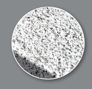
The building material "aircrete" is commonly known as aerated concrete. Aircrete is a solid building material with porous microstructures; the building material has a lot of pores (air pockets) and a low compressive strength. Aircrete has the disadvantage that it takes on moisture a lot quicker than it releases it; as such, external walls made from aircrete must always be covered with a layer of plaster or a different "skin".
