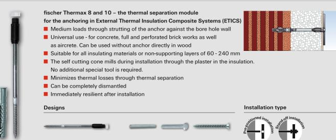
$\label{eq:thermax} Thermax 8 and 10 \mbox{ for the use with chipboard screws 4.5-6.0 mm, self-tapping screws 6.3 mm and metric screws M6/M8/M10.$
